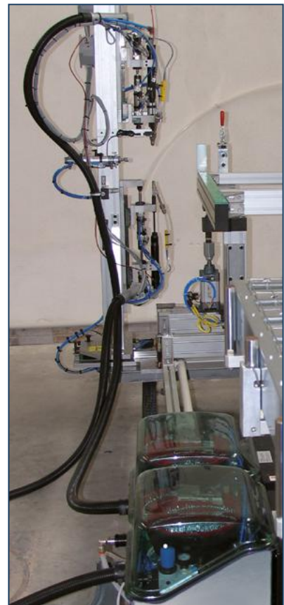
Example of multiple MCA for shutters field: assembly from the top towards the bottom and from bottom towards the top
