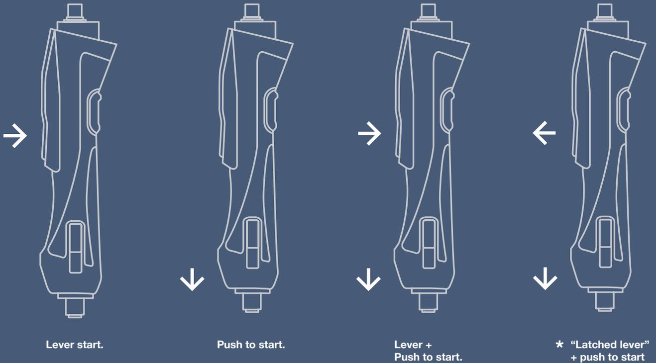
\* The "latched lever" + push to start mode allows the screwdriver to work without need to keep the lever pressed. For safety, the screwdriver activates only when pushing on the bit. In this mode, the first pressure applied to the lever starts the screwdriver until clutch shuts off, whereas a second pressure can eventually stop it before the working cycle is completed.
